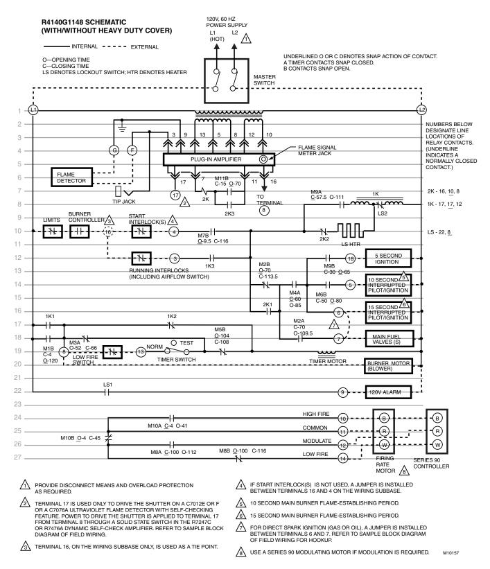
Fig. 13. Simplified schematic diagram of R4140G1148 Programmer.
